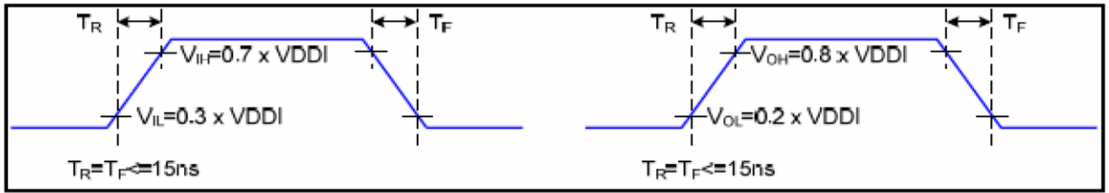
Figure 2 Rising and Falling Timing for I/O Signal
