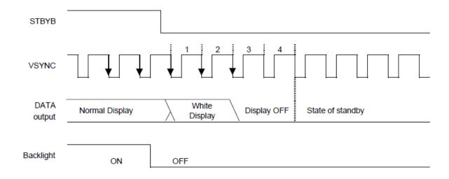
Similarly, the time of nine frames will be needed by the time a usual display is begun from the standby release by the STBYB signal. Please begin outputting in the 8th frame on the Display Data.
