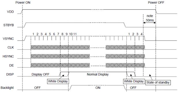
Note: For Power OFF, please turn off VDD since 50msec after the standby state shifts. When CLK and the VSYNC signal are stopped or the power supply is turned off to a regulated frame or less, the afterimage might remain.
