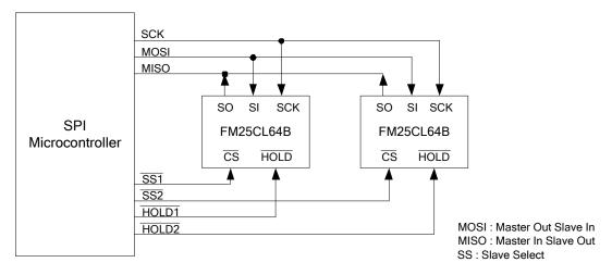
Figure 2. System Configuration with SPI port
