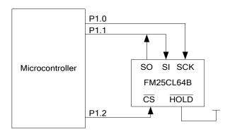
Figure 3. System Configuration without SPI port
