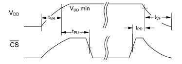
**Power Cycle Timing**  $(T_A = -40^{\circ} \text{ C to} + 85^{\circ} \text{ C}, V_{DD} = 2.7 \text{ V to } 3.65 \text{ V unless otherwise specified})$
