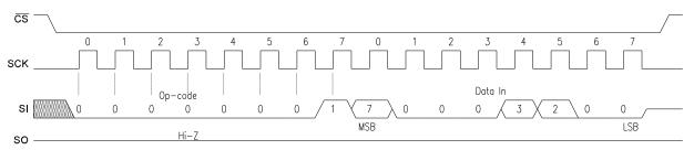
Figure 8. WRSR Bus Configuration (WREN not shown)
