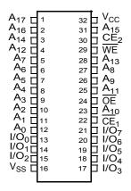
Figure 4. 32-pin STSOP (Top View)
