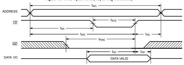
Figure 11. Write Cycle No. 3 (WE Controlled, OE LOW) [27, 30]
