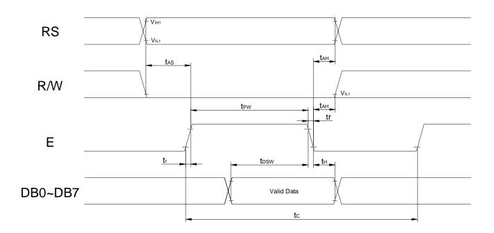
10-2-2 Read Mode (Reading Data from module to MPU)
