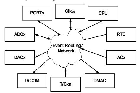
Figure 9-1. Event system block diagram.
