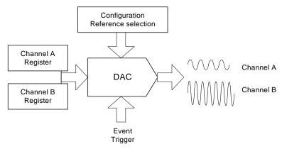
Each DAC has one continuous output with high drive capabilities for both resistive and capacitive loads. It is also possible to split the continuous time channel into two Sample and Hold (S/H) channels, each with separate data conversion registers.
