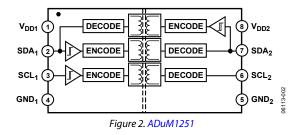
Both the ADuM1250 and the ADuM1251 contain hot swap circuitry to prevent glitching data when an unpowered card is inserted onto an active bus.
