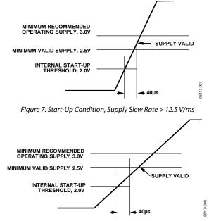
Figure 8. Start-Up Condition, Supply Slew Rate < 12.5 V/ms
