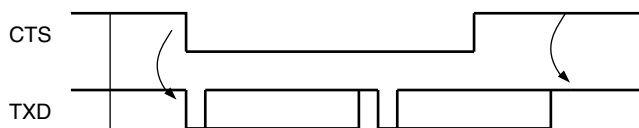
Figure 34-29. Transmitter Behavior when Operating with Hardware Handshaking
