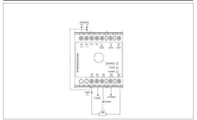
Note: Control input shall be connected either to A1-A2 or A1-A3 or A1-A4 or A1-A3-A5 in case an external potentiometer is used.
