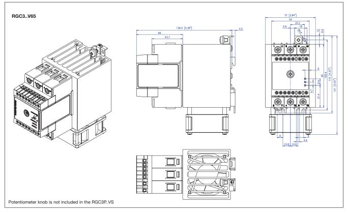
Dimensions in mm. Housing width tolerance +0.5mm, -0mm as per DIN43880. All other tolerances  $\pm 0.5\text{mm}$
