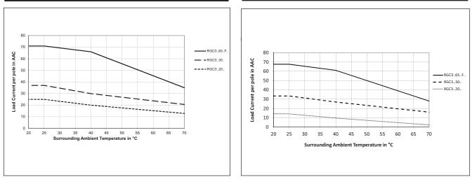
Note: Versions that utilise 24 VAC external supply (Us) are limited to a maximum operating temperature of 60°C (140°F)
