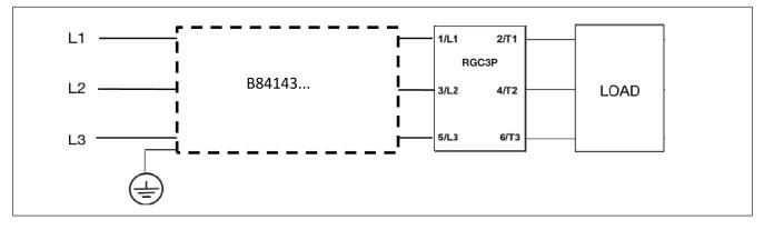
Note: The suggested filtering is determined by tests carried out on a representative setup and load. The RGC3P. is intended to be integrated within a system where conditions may differentiate from conditions utilised for tests, such as load, cable lengths and other auxiliary components that may exist within the end system. It shall be the responsibility of the system integrator to ensure that the sytsem containing the above component complies with the applicable rules and regulations.
