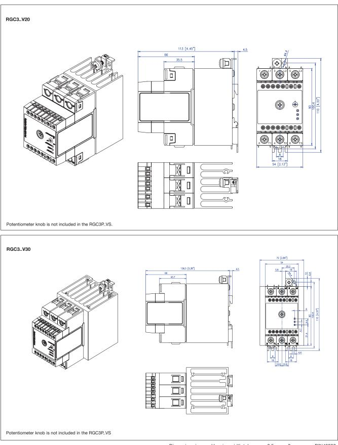
Dimensions in mm. Housing width tolerance +0.5mm, - 0mm as per DIN43880. All other tolerances  $\pm 0.5\text{mm}$
