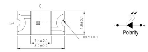
For reflow soldering
