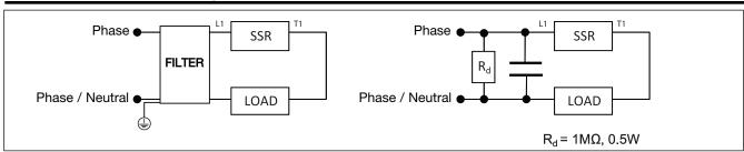
Note: The suggested filtering is determined by tests carried out on a representative setup and load. The RGC1P. is intended to be integrated within a system where conditions may differentiate from conditions utilised for tests, such as load, cable lengths and other auxiliary components that may exist within the end system. It shall be the responsibility of the system integrator to ensure that the sytsem containing the above component complies with the applicable rules and regulations.
