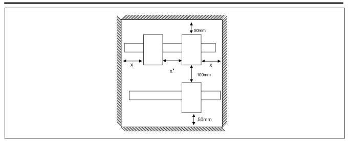
$<sup>^{\</sup>star}$  Refer to Current Derating vs spacing curves. Spacing between SSR and panel walls should be >5mm.
