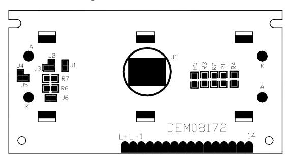
Note: In application module, R1~R4=4.7 k $\Omega$  , R5=75k $\Omega$
