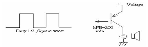
The base current Ib should high enough so that it saturates the collector current of the transistor with the CB load.
