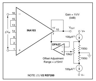
FIGURE 4. Output Offsetting.
