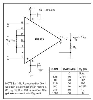
FIGURE 1. Basic Circuit Configuration.
