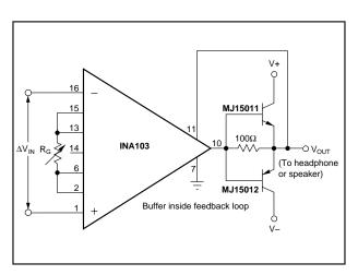
FIGURE 11. Increasing Output Circuit Drive.
