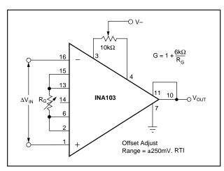
FIGURE 3. Offset Adjustment Circuit.
