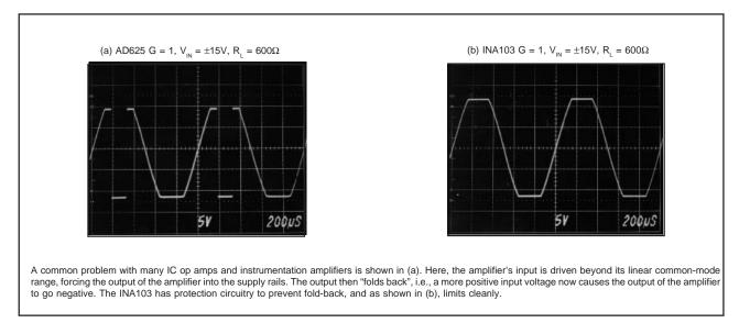
FIGURE 9. INA103 Overload Condition Performance.
