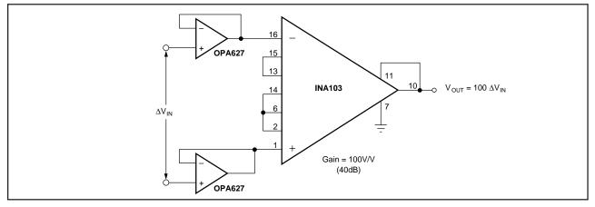
FIGURE 14. Gain-of-100 INA103 with FET Buffers.
