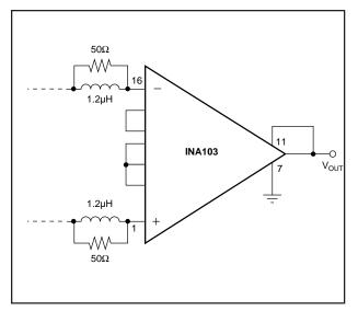
FIGURE 2. Input Stabilization Network.
