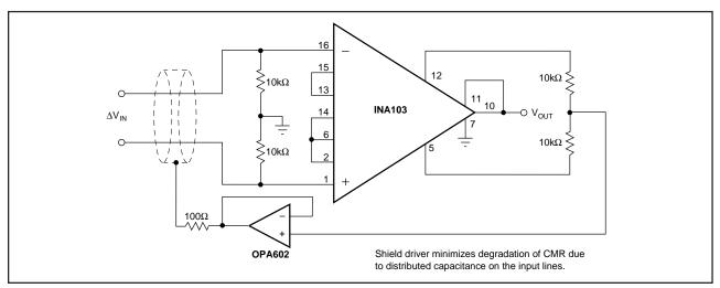
FIGURE 13. Instrumentation Amplifier with Shield Driver.
