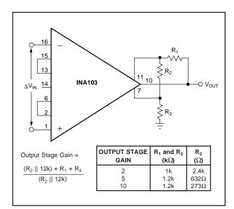
FIGURE 7. Gain Adjustment of Output Stage.
