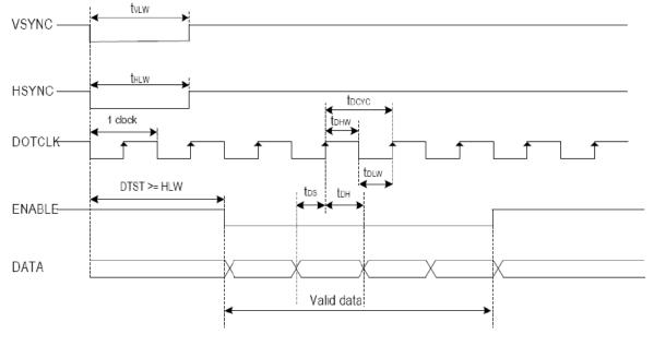
DTST: Setup Time for Data Transmission
