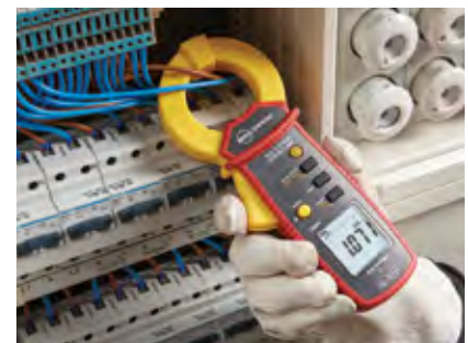
Differential current measurement with leakage current clamp
