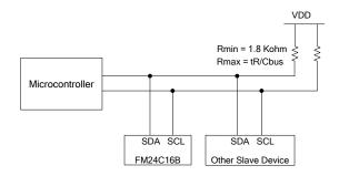
Figure 2. Typical System Configuration
