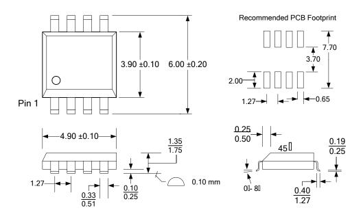
Refer to JEDEC MS-012 for complete dimensions and notes. All dimensions in  $\underline{\text{millimeters}}$ .
