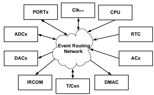
Figure 9-1. Event System Block Diagram
