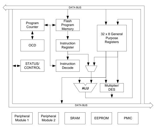
The AVR uses a Harvard architecture - with separate memories and buses for program and data. Instructions in the program memory are executed with a single level pipeline. While one instruction is being executed, the next instruction is pre-fetched from the program memory. This
