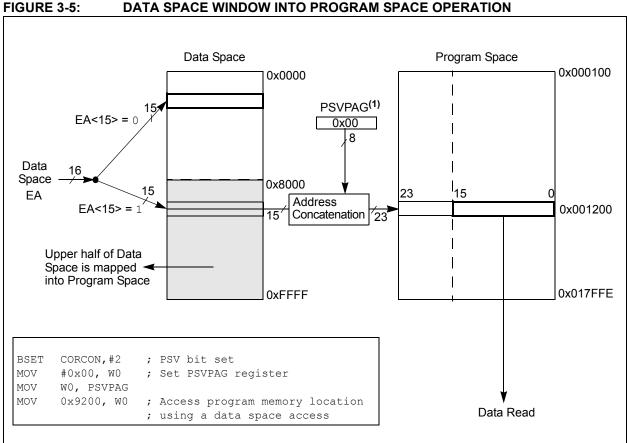
**Note:** PSVPAG is an 8-bit register, containing bits <22:15> of the program space address (i.e., it defines the page in program space to which the upper half of data space is being mapped).
