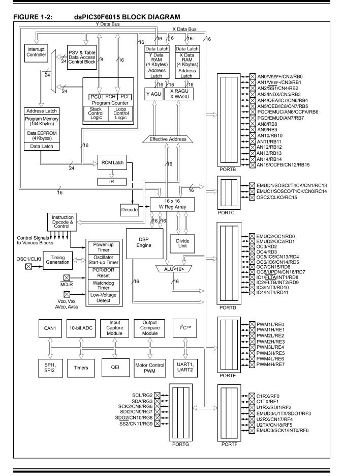
Table 1-1 provides a brief description of the device I/O pinout and the functions that are multiplexed to a port pin. Multiple functions may exist on one port pin. When multiplexing occurs, the peripheral module's functional requirements may force an override of the data direction of the port pin.
