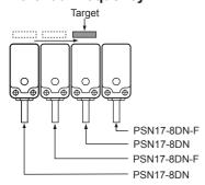
When installing several proximity sensor closely, it may cause malfunction due to mutual interference. Therefore, please use differential frequency for the application \*\*Differential frequency type is only for 17 square.
