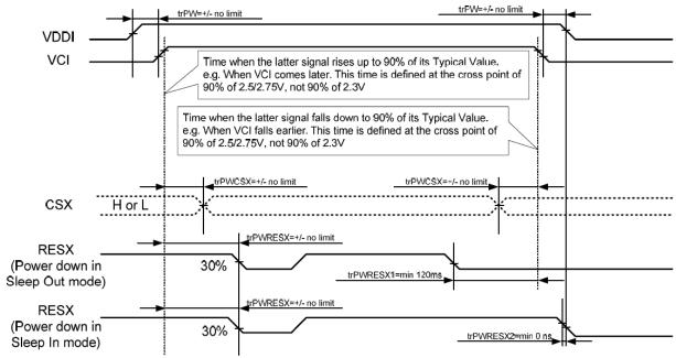
trPWRESX1 is applied to RESET (RESX) falling in the Sleep Out Mode trPWRESX2 is applied to RESET (RESX) falling in the Sleep In Mode
