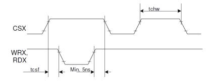
Write to read or read to write timings [WR (WRX), RD (RDX)]:
