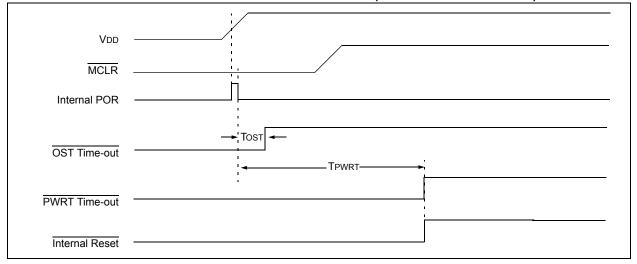
FIGURE 20-5: TIME-OUT SEQUENCE ON POWER-UP (MCLR NOT TIED TO VDD): CASE 2
