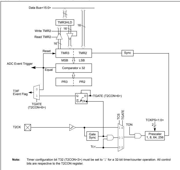
FIGURE 10-2: 16-BIT TIMER2 BLOCK DIAGRAM
