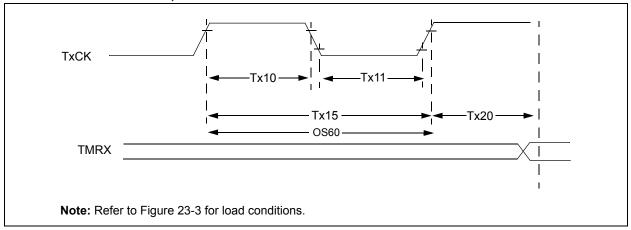
TABLE 23-23: TYPE A TIMER (TIMER1) EXTERNAL CLOCK TIMING REQUIREMENTS<sup>(1)</sup>
