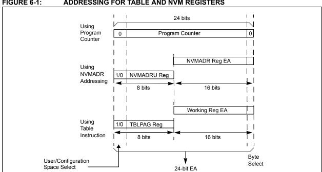
FIGURE 6-1: ADDRESSING FOR TABLE AND NVM REGISTERS
