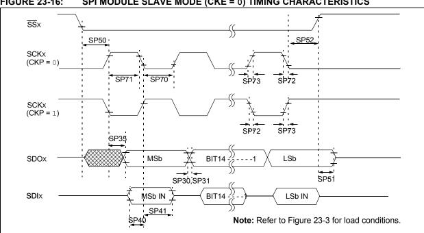
FIGURE 23-16: SPI MODULE SLAVE MODE (CKE = 0) TIMING CHARACTERISTICS
