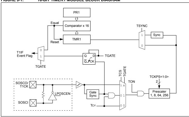
FIGURE 9-1: 16-BIT TIMER1 MODULE BLOCK DIAGRAM
