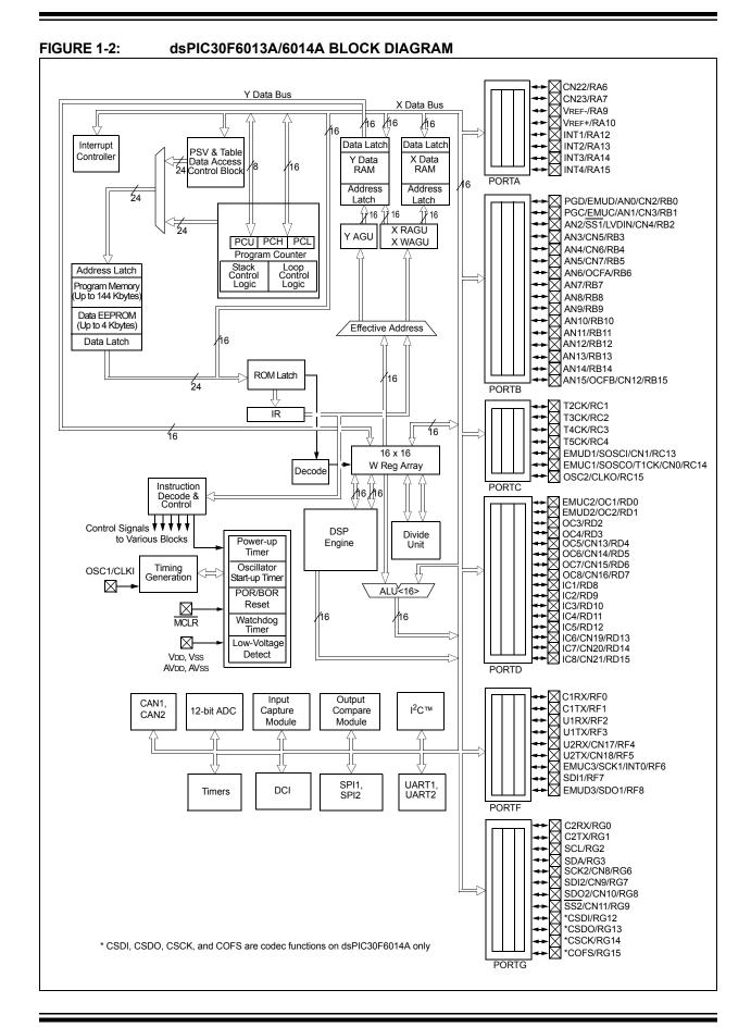
Table 1-1 provides a brief description of device I/O pinouts and the functions that may be multiplexed to a port pin. Multiple functions may exist on one port pin. When multiplexing occurs, the peripheral module's functional requirements may force an override of the data direction of the port pin.
