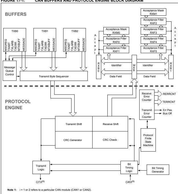
**FIGURE 17-1:** CAN BUFFERS AND PROTOCOL ENGINE BLOCK DIAGRAM
