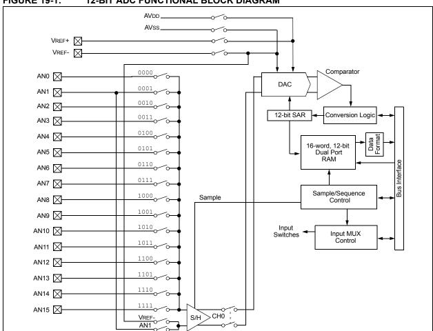
FIGURE 19-1: 12-BIT ADC FUNCTIONAL BLOCK DIAGRAM
