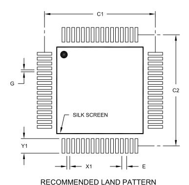
Units **MILLIMETERS** NOM **Dimension Limits** MIN MAX 0.50 BSC Contact Pitch Е 11.40 Contact Pad Spacing C1 C2 Contact Pad Spacing 11.40 0.30 Contact Pad Width (X64) X1 Contact Pad Length (X64) <u>Y1</u> 1.50 Distance Between Pads G 0.20
