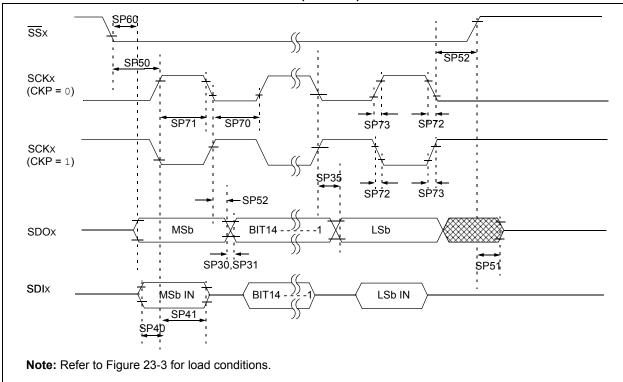
TABLE 23-34: SPI MODULE SLAVE MODE (CKE = 1) TIMING REQUIREMENTS
