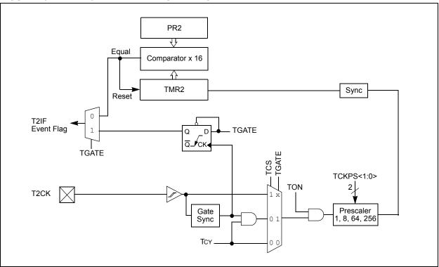
FIGURE 10-3: 16-BIT TIMER3 BLOCK DIAGRAM
