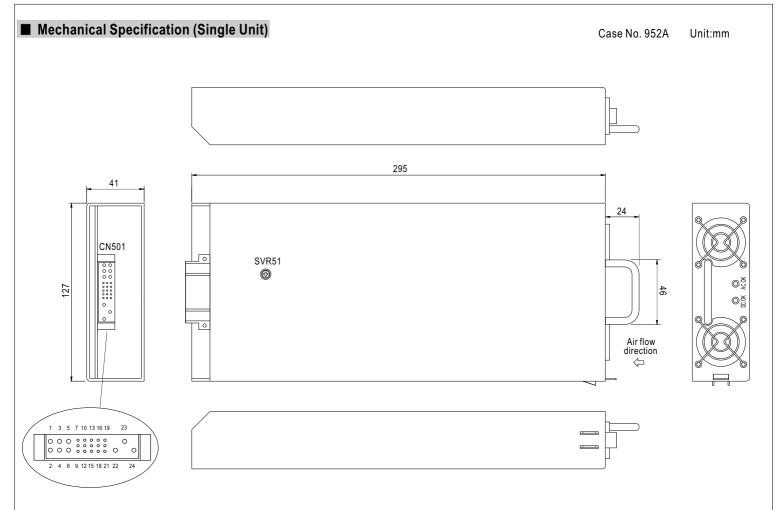
Input / Output Connector Pin No. Assignment(CN501): Postronic PCIB24W9M400A1
