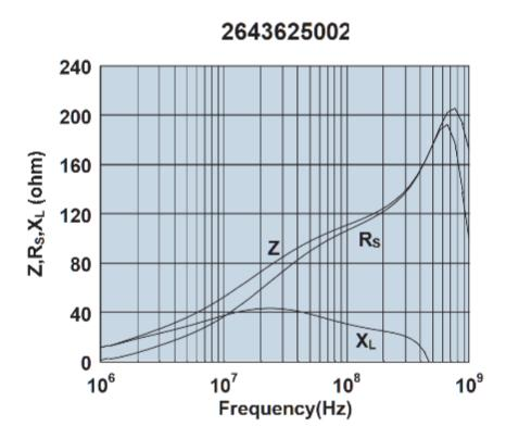
Impedance, reactance, and resistance vs. frequency.
