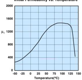
Measured on a 17/10/6mm toroid at 100kHz.
