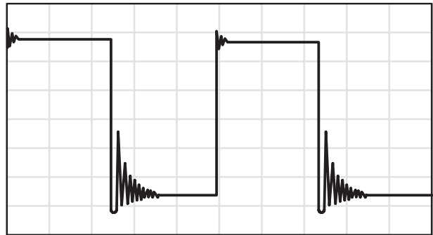
(b) C_L = 260 \text{ pF} , R_L = \text{NO LOAD}
