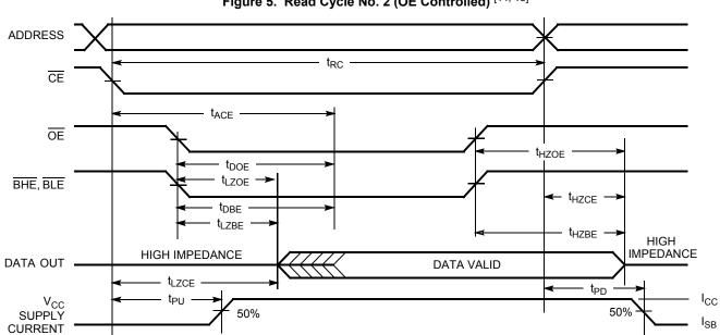
Figure 5. Read Cycle No. 2 (OE Controlled) <sup>[14, 15]</sup>
