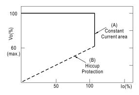
Typical LED power supply I-V curve
