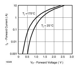
Figure 2. Forward Current vs. Forward Voltage
