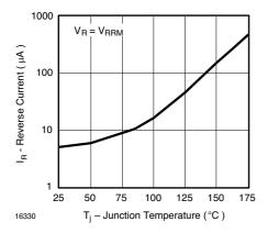
Figure 4. Reverse Current vs. Junction Temperature
