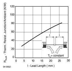
Figure 1. Max. Thermal Resistance vs. Lead Length
