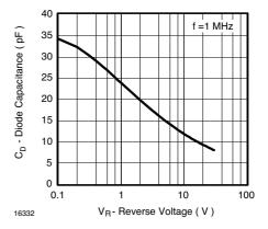
Figure 6. Diode Capacitance vs. Reverse Voltage
