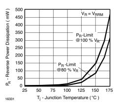
Figure 5. Max. Reverse Power Dissipation vs. Junction Temperature
