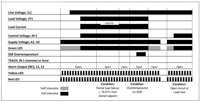
Upon application of supply voltage, the yellow and red LED will flash continuously in sequence (i.e., scroll) indicating that the device has no current setpoint stored. The green LED is ON at half intensity indicating the presence of supply voltage. As soon as control voltage is applied the green LED will be ON at full intensity. The alarm output, which is normally closed, is open to indicate that the SSR has no stored setpoint.
