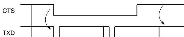
Figure 36-29. Transmitter Behavior when Operating with Hardware Handshaking
