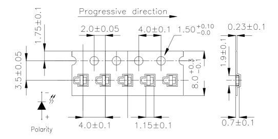
**Note:** The tolerance unless mentioned is  $\pm 0.1$ mm, unit is mm.
