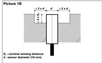
Quasi-flush mountable proximity switches, when installed together in damping material, must be according to Picture
