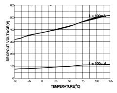
Figure 7. Dropout Voltage
