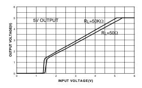
Figure 2. Dropout Characteristics
