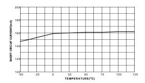
**Figure 6. Short Circuit Current**
