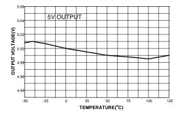
Figure 5. Output Voltage vs. Temperature
