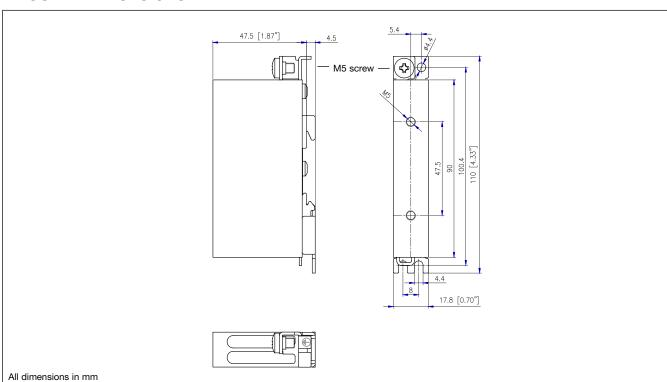
Note: M5 PE screw not provided with SSR. Maximum mounting torque 1.5Nm (13.3 in-lb).
