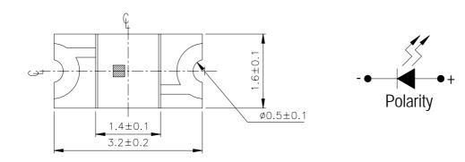
For reflow soldering
