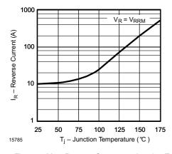
Figure 2. Max. Reverse Current vs. Junction Temperature
