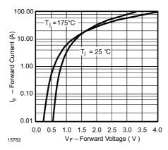
Figure 5. Max. Forward Current vs. Forward Voltage
