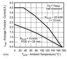
Figure 4. Max. Average Forward Current vs. Ambient Temperature
