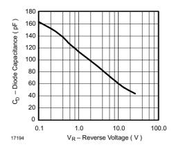
Figure 3. Diode Capacitance vs. Reverse Voltage
