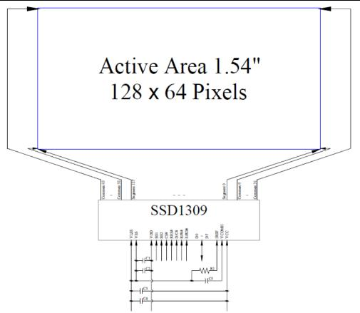
MCU Interface Selection: BS1 and BS2 Pins connected to MCU interface: CS#, RES#, D/C#, R/W#, E/RD#, and D0~D7
