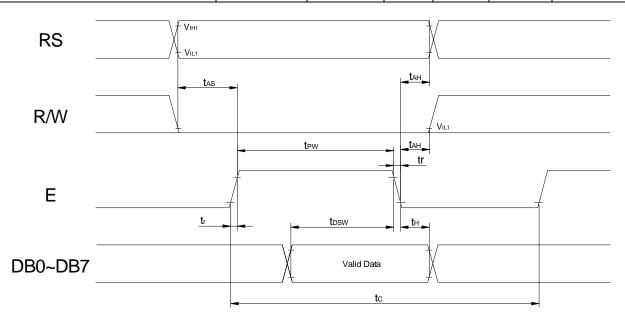
10-2-2 Read mode (reading data from MPU to module)
