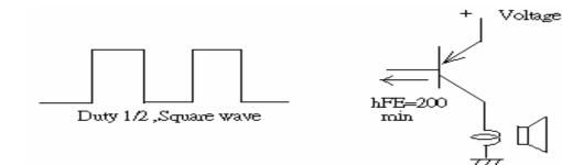
The base current Ib should high enough so that it saturates the collector current of the transistor with the CB load.
